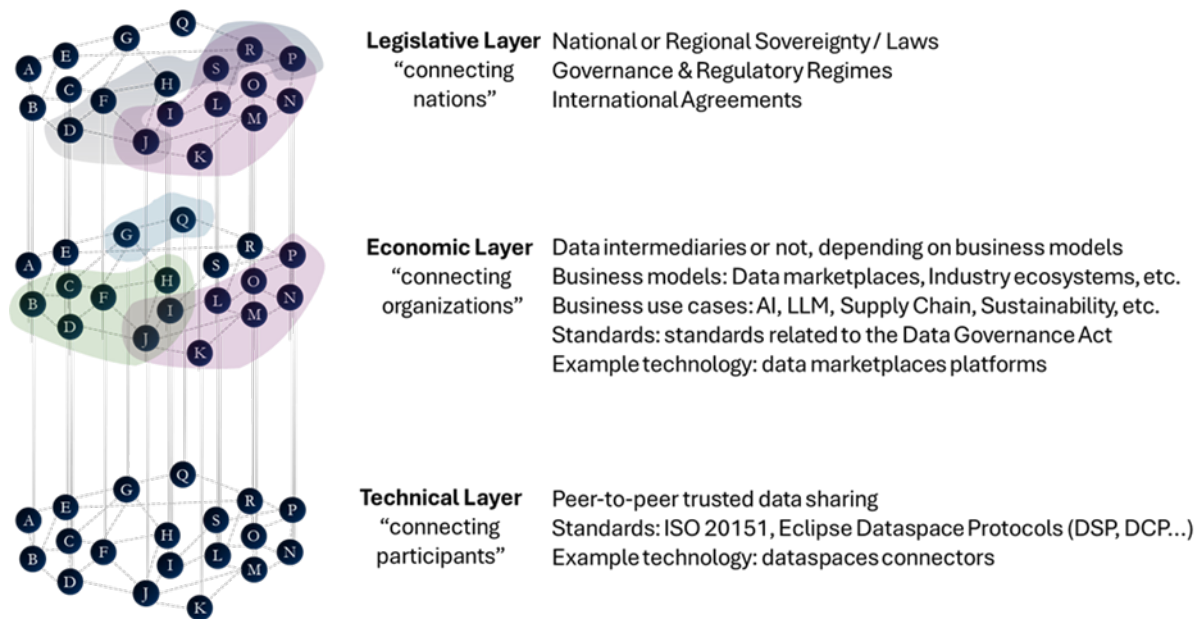
Figure 10: Layers of a data space
